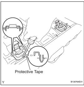
(b) Using a screwdriver with its tip wrapped in protective tape, disengage the 3 claws and remove the tether anchor cover.
