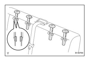
(b) Disengage the 2 claws and remove the rear seat headrest support.
